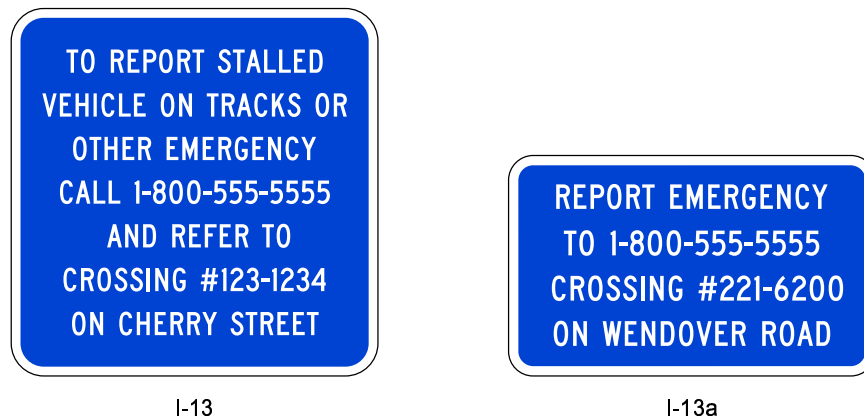
Figure 10C-4. Examples of Emergency Notification Signs
