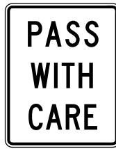
Figure 2B-8. Passing, Keep Right, and Truck Lane Signs
