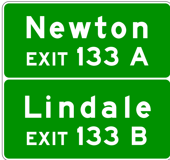
Figure 2E-17. Supplemental Guide Signs for Multi-exit Interchanges
